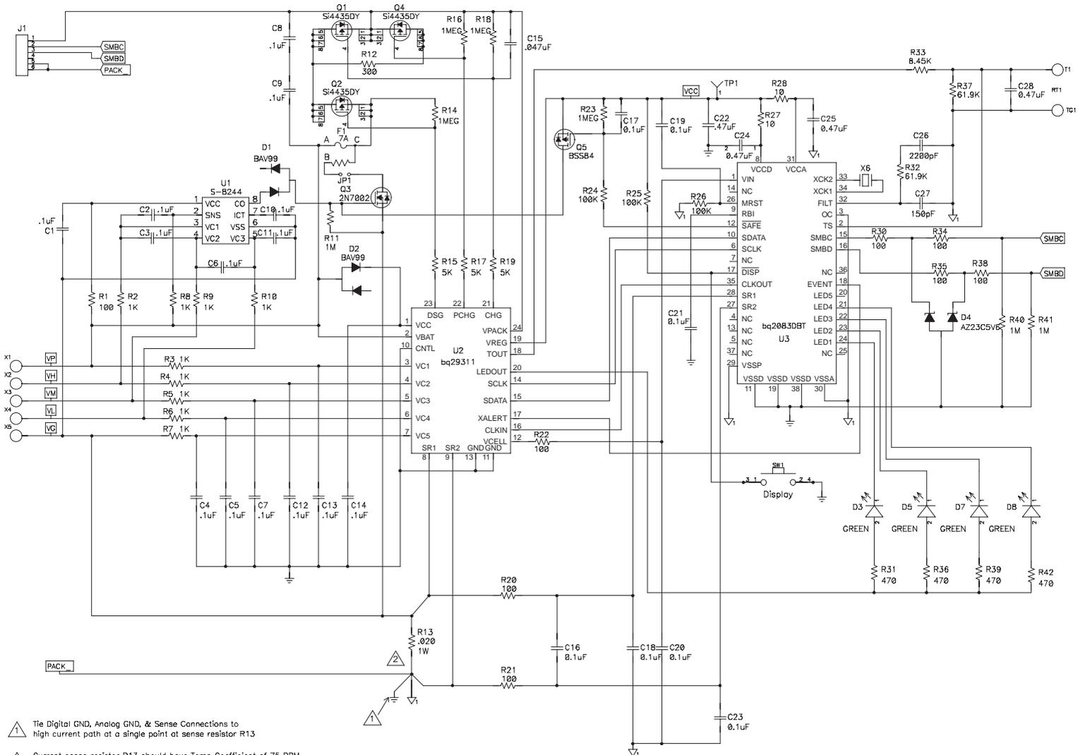
1 Tie Digital GND, Analog GND, & Sense Connections to high current path at a single point at sense resistor R13
